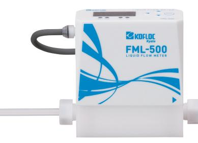
The FML-500 is a straight tube type ultrasonic flow meter for liquids. A new PFA material with excellent chemical resistance is used for parts in contact with the liquid, and the simple straight design facilitates maintenance without any obstacles inside the tube. It comes with a built-in display and the flow rate can be measured by connecting it to a power source. Flow rates up to a full scale of 5 L/min can be measured with high accuracy.
