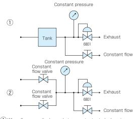
When flows are discharged at a constant rate by keeping the tank pressure at a given level
