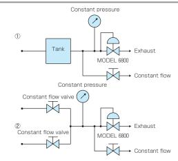
① In this example, constant flow is discharged, while the tank inside pressure is kept con-
